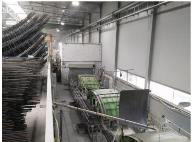
The segment cladding is produced and stored in an on-site casting facility using a carousel system. Source: GKI Maria Stein consortium
