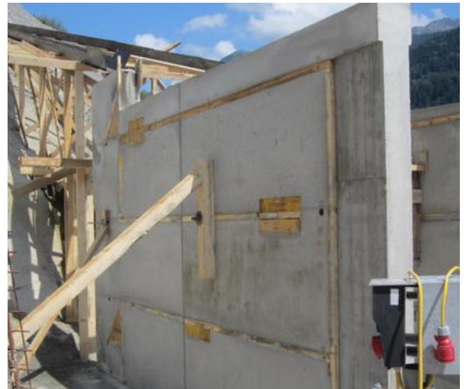
In the TB Stams concrete factory, a large-scale test was carried out to find a suitable concrete recipe for the concrete backfill. Source: GKI PRB consortium
