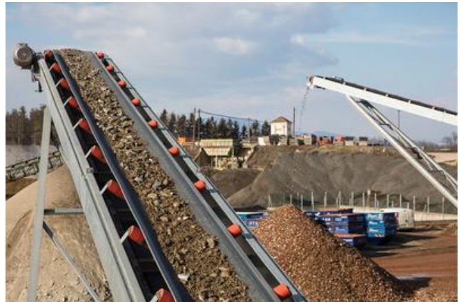
Conveyor belts with medium fraction and the end product. Source: Daniel Ulbricht-Sundt
