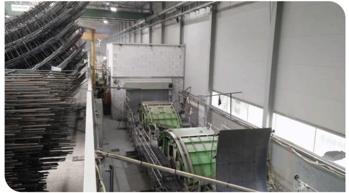
The segment cladding is produced and stored in an on-site casting facility using a carousel system. Source: GKI Maria Stein consortium
