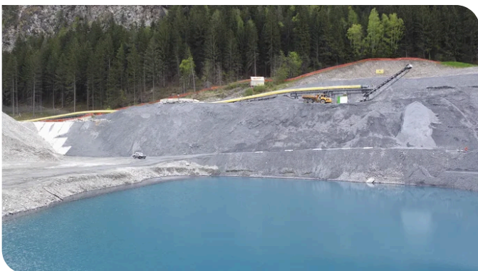
Aggregate material is collected from a side entrance and processed on site. Source: GKI Maria Stein consortium
