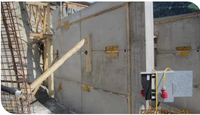
In the TB Stams concrete factory, a large-scale test was carried out to find a suitable concrete recipe for the concrete backfill. Source: GKI PRB consortium
