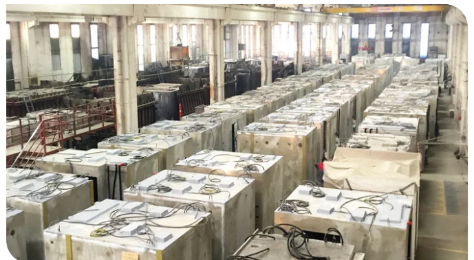
Production of the prefabricated bathroom cells made of reinforced concrete. Picture: PORR AG
